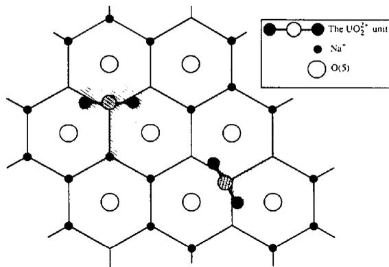
Fig. 5. Two possible environments for the UO<sub>2</sub><sup>2+</sup> unit in the conduction plane.
